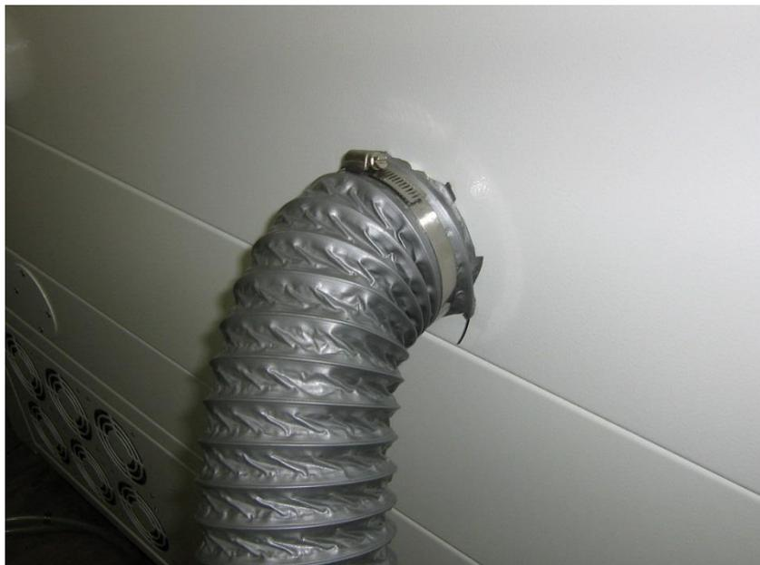
**5. Connect hose from air filter to compressor**
