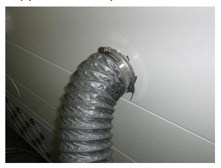
5. Connect hose from air filter to compressor
