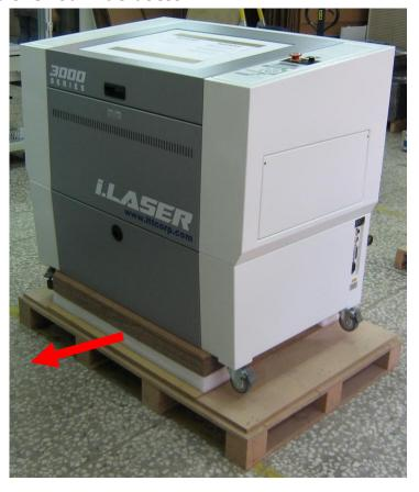
8. Place the slide board which is in the upper box and roll down the machine. (If you order slide board.)
